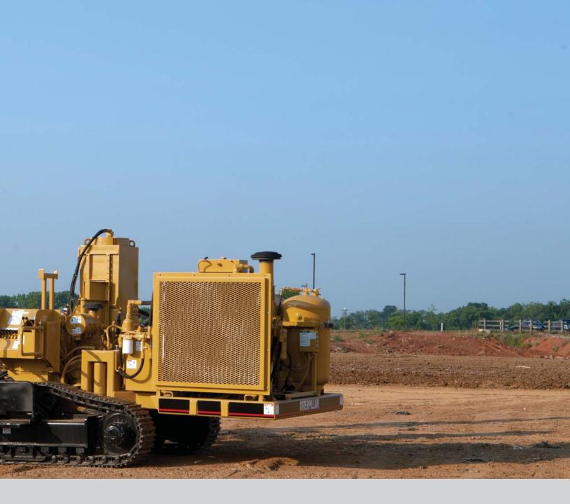
MD5090 delivers high productivity by getting more holes drilled with fewer set ups. These fast cycle times are achieved thanks to its top performing rock drill, large pattern coverage, and a power group that's ideally sized for drilling 89 mm-127 mm (3.5 in-5.0 in) holes. A non-cab, non-enclosure version, as shown, is lightweight and service accessible.
