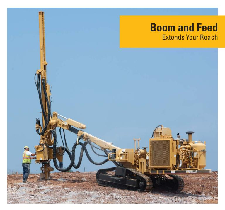
A sturdy extendible boom and feed provides excellent pattern coverage and requires fewer setups. The heavy-duty boom is constructed of thick square tubing with steel plate reinforcements in key areas to add strength. The feed system resists torsion and thrust loads because it is built with diagonally braced high strength steel channels.
