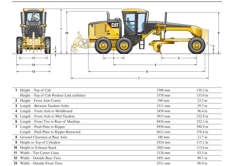
All dimensions are approximate, based on standard machine configuration with 14R24 tires.
