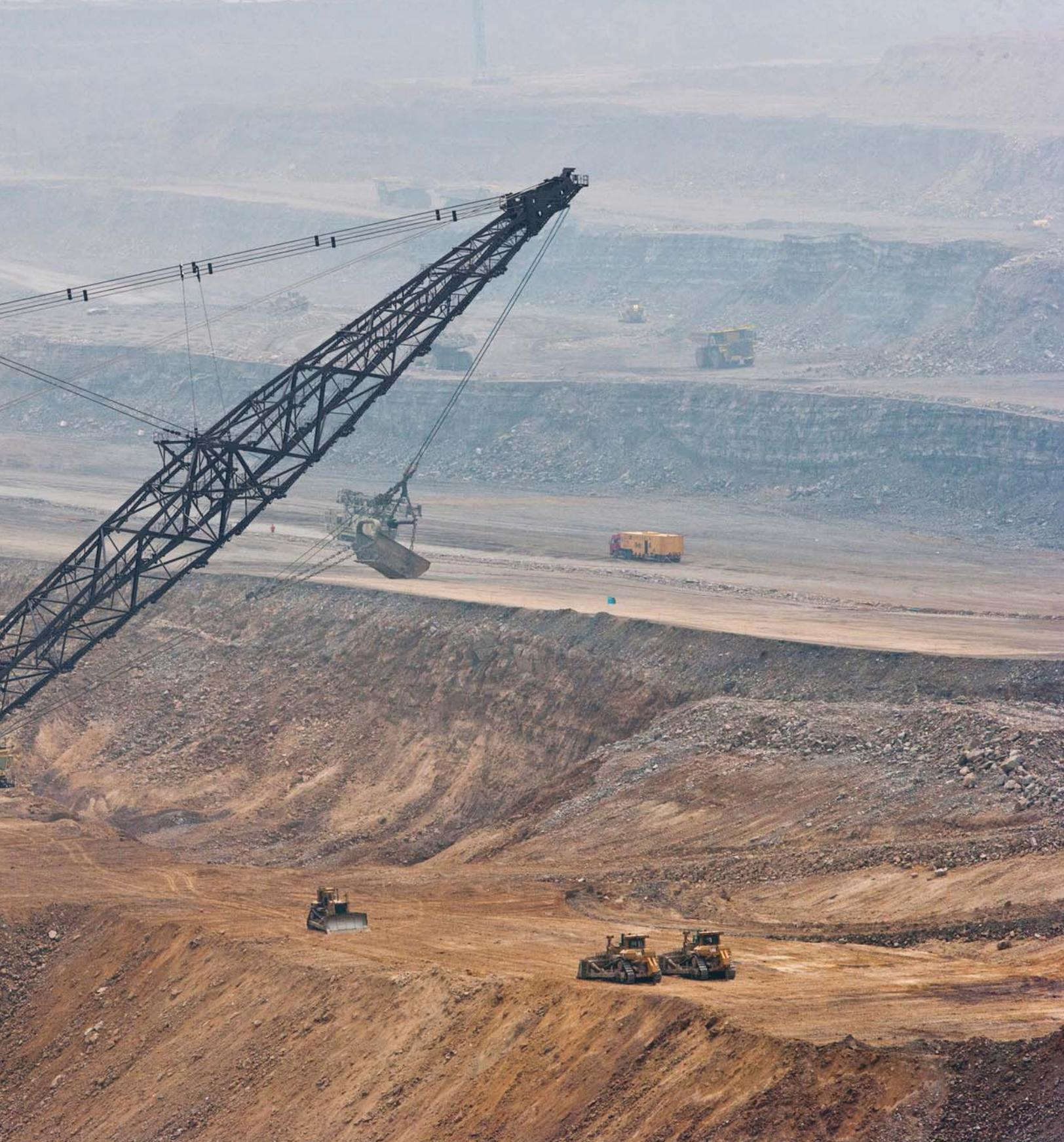
**Delivering extremely high levels of overburden removal productivity at a low cost per tonne (ton), the Cat 8200 model dragline offers all of the innovative technology of our flagship model – the Cat 8750 – but on a mid-range size scale. Along with a lower initial capital outlay compared to larger draglines, the 8200's unique combination of technology, size, and long operating life ensures the low total cost of ownership you need for a strong return on your investment.**
