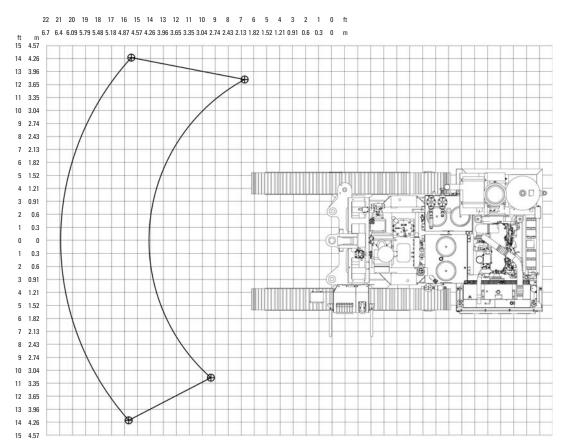
Drill more holes with fewer set-ups thanks to a sturdy boom system that is telescopic, has a 1.52 m (5 ft) extension, and swings 40 degrees to the left and right.
