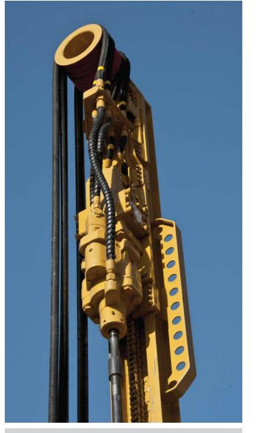
The MD5090 is equipped with the HPR4519 hydraulic powered percussion rock drill rated at 19 kW (25 hp) output energy with dual hydraulic variable rotation motors producing 908 N·m (670 lbf-ft) torque.
