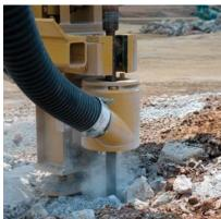
*Powered to clear holes up to 127 mm (5 in), the optional dry dust collection system effectively manages rock fragments and dust and is easy to clean and service.*
