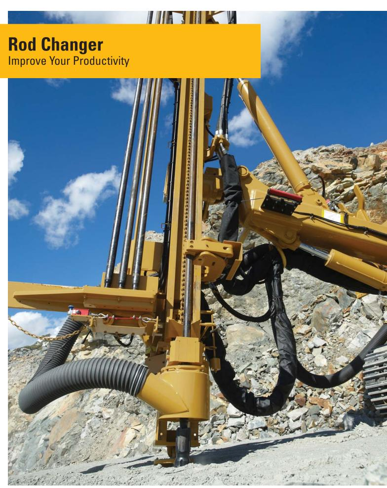
Providing you with proven versatility, the MD5125 is equipped with a sturdy rod changer that holds multiple rods allowing the boom extension to reach far and drill deep while maintaining stability. Each feed and rod changer can accommodate various lengths and diameters of drill steel. The selection and use of drill steel varies based on the desired hole depth and diameter per the blasting plan.
