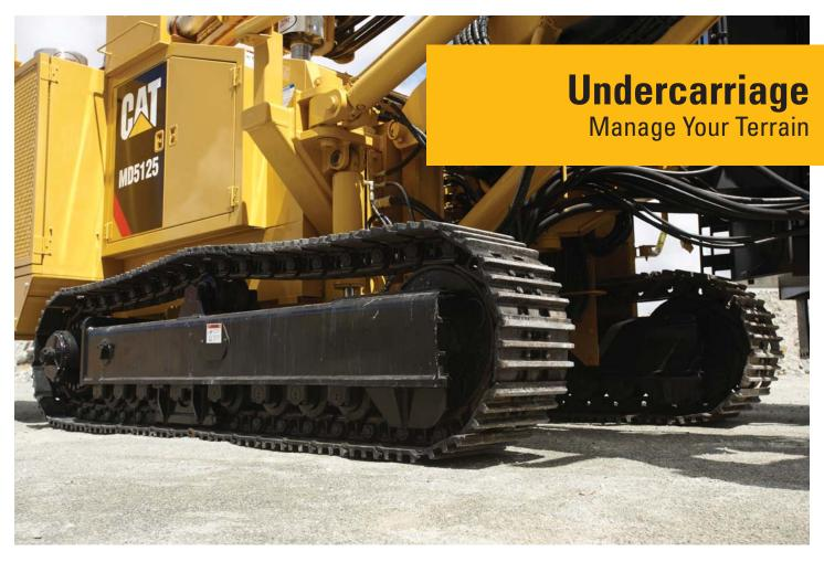
The undercarriage on the MD5125 provides excellent maneuverability thanks to its low center of gravity and high ground clearance which is beneficial in tough terrain.
