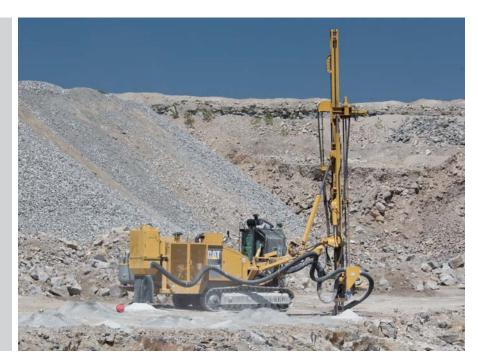
Longer boom length and feed is ideal for drilling deep holes with few rod changes. Boom is fixed and in ready position.
