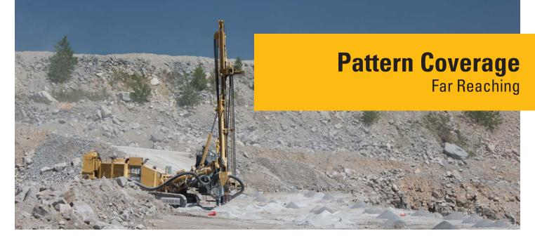
To negotiate overhead limitations or uneven terrain the 3.66 m (12 ft) feed and the heavy-duty 2.6 m (8.5 ft) telescopic boom on the MD5125 C gives a lower operating range and extends an additional 0.9 m (3 ft) when needed. The MD5125 CL is always in ready position with its non-telescopic 2.8 m (9 ft) boom.
