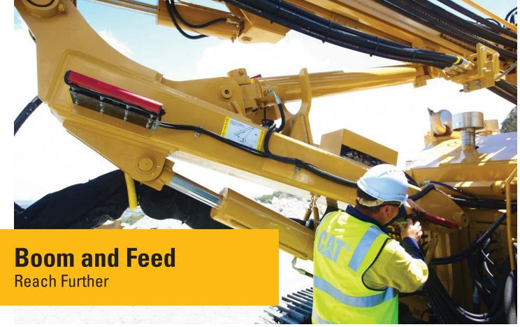
A sturdy boom and feed support the carousel rod changer providing excellent pattern coverage and fewer required setups. The heavy-duty boom is constructed of thick square tubing with steel plate reinforcements in key areas to add strength. Built with high strength steel channels with diagonal internal bracing, the feed system resists torsion and thrust loads.
