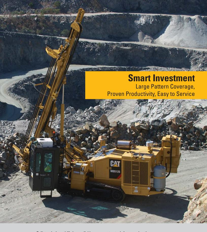
Built tough, these drills have reliable components, sturdy frames, robust booms and feeds that contribute to outstanding availability. They are designed to be easy to service with conveniences such as ground level access to all major service points and well-organized electrical and hydraulic arrangements. Available in two models MD5125 C and MD5125 CL.
