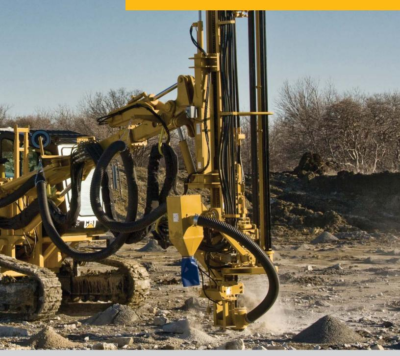
The Cat® MD5075 achieves large pattern coverage with a sturdy extendable boom and reduces your cycle time with an efficient carousel rod changer. Its powerful rock drill, durable Cat components, and ease of maintenance contribute to the exceptional value of this proven machine.
