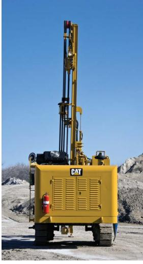
Our proven and reliable undercarriage is designed to tram challenging terrain. Your operator can quickly and precisely position the MD5075 thanks to its low center of gravity and high ground clearance.
