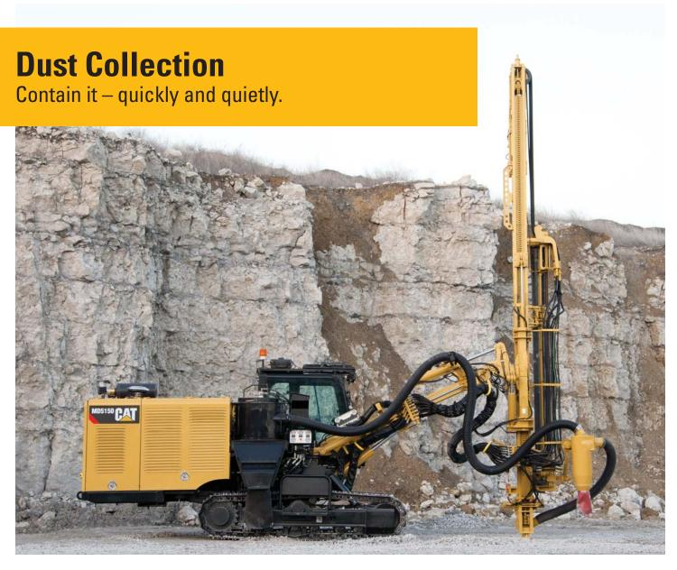
Powered to clean holes up to 152 mm (6 in), the MD5150 dry dust collection system is efficient, quiet and it consumes less power than traditional dust collectors. The heavy-duty system effectively manages rock fragments and dust yet is also easy to clean and service.
