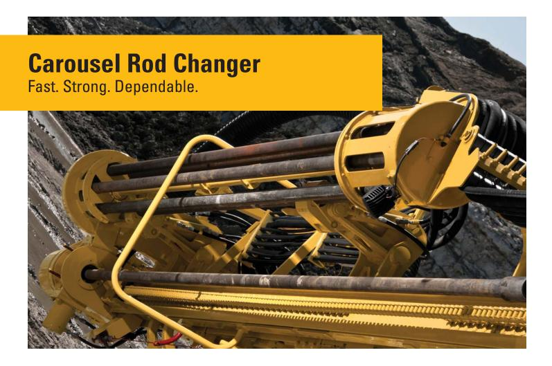
To improve your overall productivity, our new carousel rod changer significantly reduces rod change time. Additionally the carousel is supported by a sturdy feed and the extension boom allowing for large pattern coverage so fewer set ups are required.
