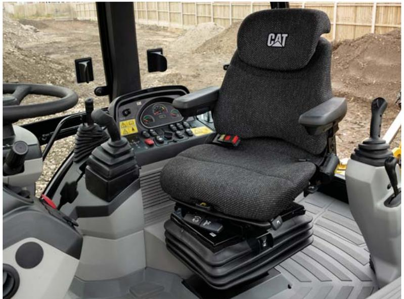
The 432F cab is designed with today's operator in mind. The design provides maximum comfort, ease of operation and with modern styling, meets the requirements of today's demanding operator. The design incorporates curved glass for improved interior space and visibility. A wide cab provides a spacious environment for better performance when turning the seat from one mode of operation to the other. Cab comfort is enhanced with the first-class Cat air suspension seat, reducing fatigue.
