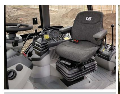
The 428F Cab is designed with today's operator in mind. The design provides maximum comfort, ease of operation and with modern styling, meets the requirements of today's demanding operator. The design incorporates curved glass for improved interior space and visibility. A wide cab provides a spacious environment for better performance when turning the seat from one mode of operation to the other. Cab comfort is enhanced with the first-class Cat air suspension seat, reducing fatigue.
