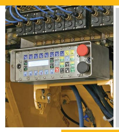
Caterpillar manufactures a complete range of shield support control systems ranging from manual hydraulic controls to the highly acclaimed PMC-R electronic control system for the most advanced face automation and equipment monitoring.
