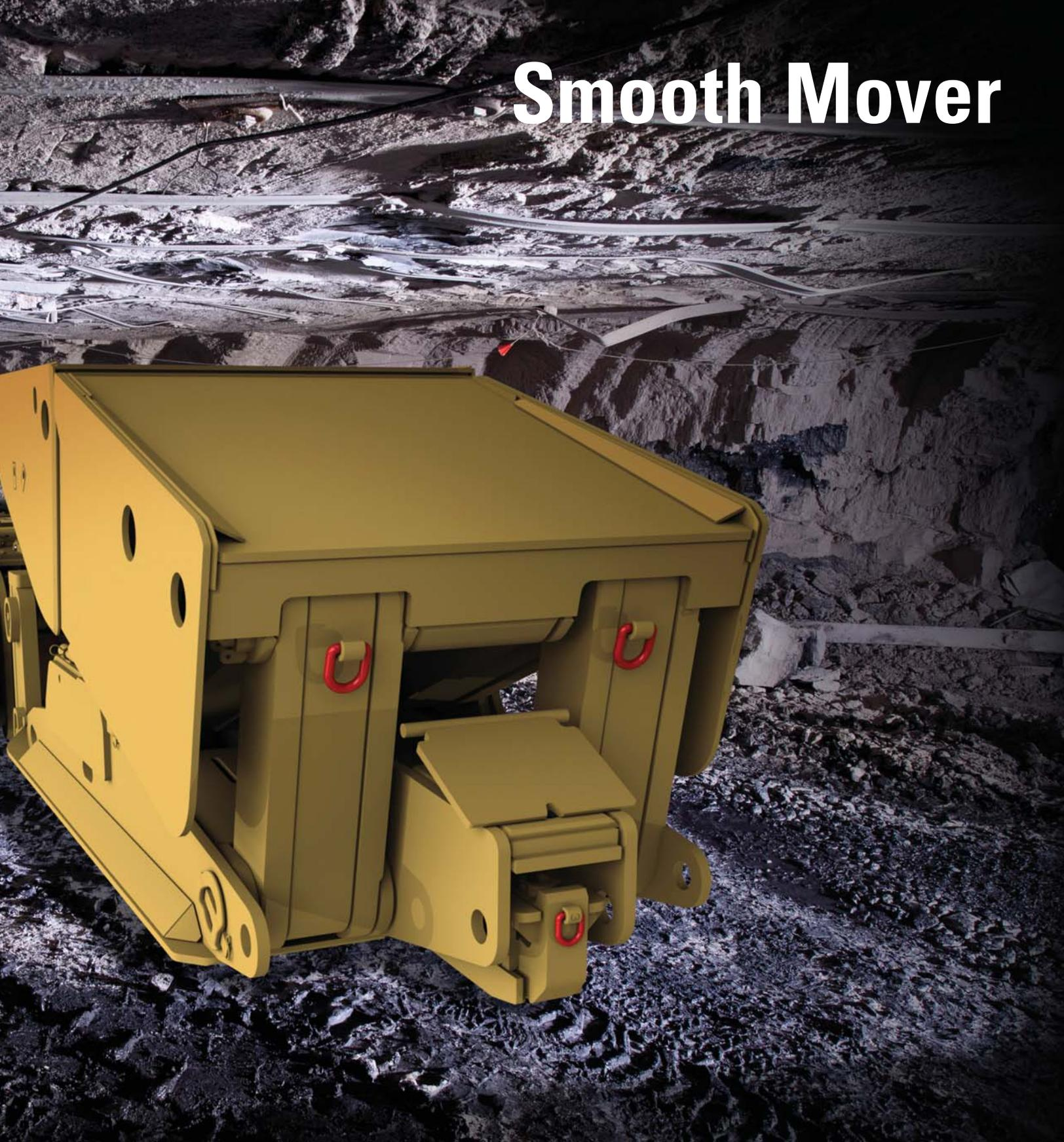
Longwall moves represent an enormous challenge to underground transportation logistics. Caterpillar offers a full range of roof support carriers to meet the needs of efficient longwall moves. With an increased lift capacity of 45 tonnes (50 ton), the SH650 can handle almost any piece of longwall equipment in a move. In addition to enhanced traction and maneuverability, the SH650 offers improved range of motion of the lift, allowing easier load engagement.
