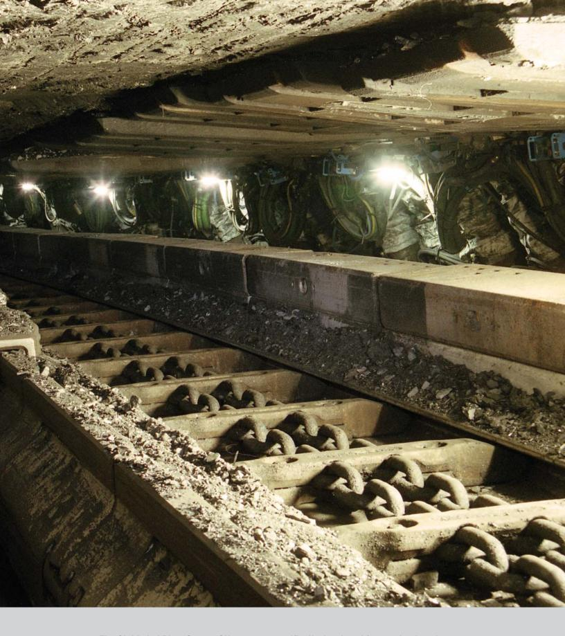
The Gleithobel Plow System GH1600 was specifically developed for very hard coal and high productivity by doubling the installed power of the GH800 to 1600 kW (1,080 hp). It can be used in seams from approximately 1.0 m (39 in) up to 2.53 m (91 in) with a portal arm.
