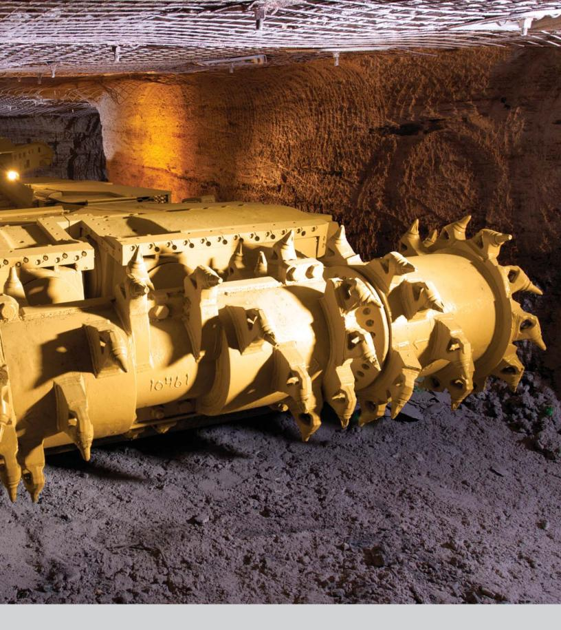
Weighing in at 61.2 tonnes (135,000 lb) and with a compact design specifically for low- to mid-seam operations, the Cat CM235 continuous miner incorporates all the robust features of the CM200 Series plus new features and enhancements. With  $2 \times 205$  kW ( $2 \times 275$  hp) cutter-head motors, it is the most powerful continuous miner in its class.
