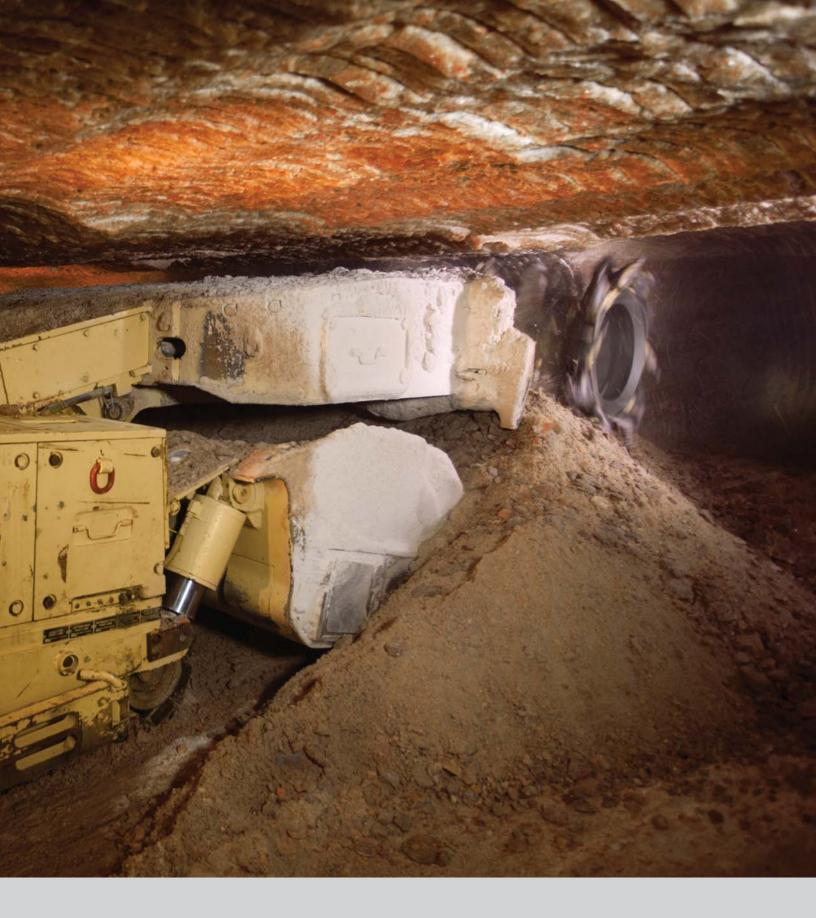
The Cat® CM445 Continuous Miner is designed for mining applications ranging from 1626 mm (64 in) up to 3810 mm (150 in) where increased weight to horsepower ratios are required for performance in hard cutting type mining conditions. The hard head-style cutter head makes the CM445 the preferred miner for hard-cutting coal, trona, and potash.
