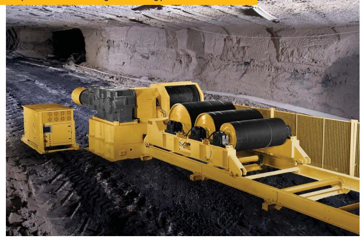
Increase conveyor efficiency at your operation with our responsive tensioning technology. Caterpillar engineered take-ups and storage units apply continuous and accurate belt tension supporting slack removal and efficient conveyor operation.
