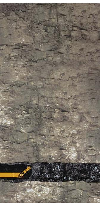
Highwall mining is a proven primary method for mining coal from exposed seams. In this method of mining, an unmanned cutter module is driven underground and operated in front of the highwall.
