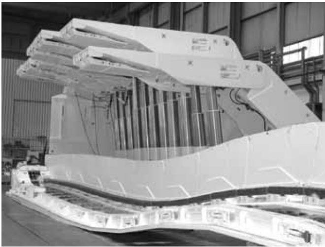
Vertical bending capability of Cat face conveyor systems
