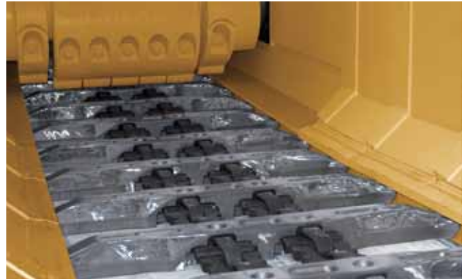
PowerChain inside a Cat BSL in the crusher area
