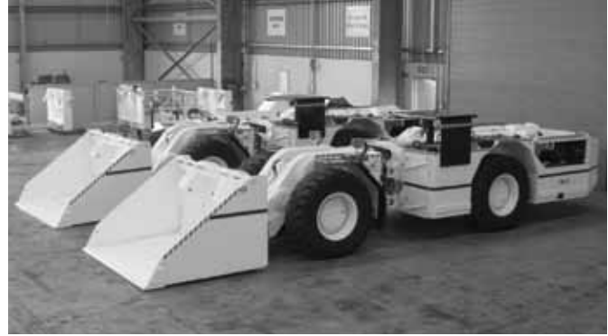
CL10 compact loader with RAS bucket attached
