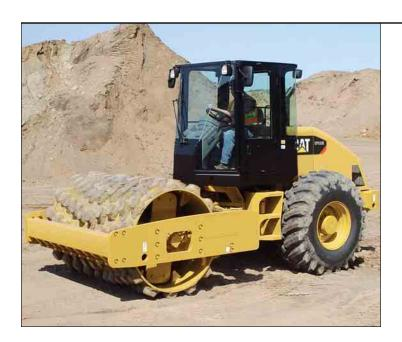
**Padfoot drum.** The padfoot drum has 140 pads welded on the drum in a chevron arrangement.
