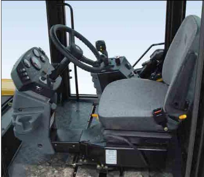
**Seat.** The comfortable and durable seat has adjustable fore/aft position, suspension stiffness and flip-up arm rests with a 76 mm wide retractable seat belt.
