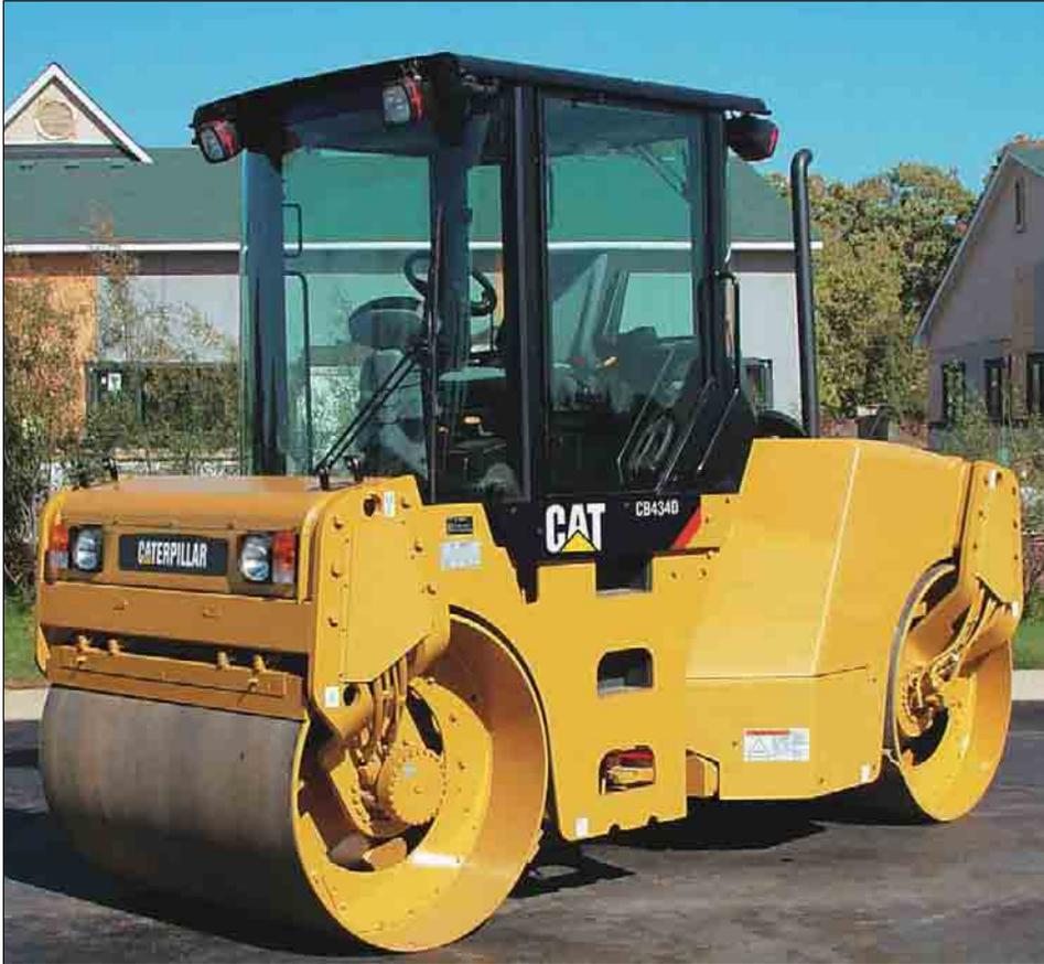
**Hood arrangement.** Vertical-lift hood arrangement allows routine service when parked close to other machines and structures.
