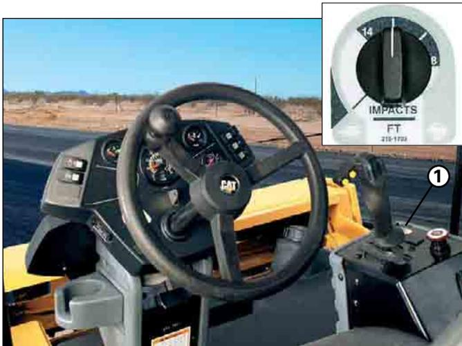
**Cab option.** The optional cab is a spacious and comfortable work environment with more interior room, better ergonomics and a dramatic reduction in interior sound levels.
