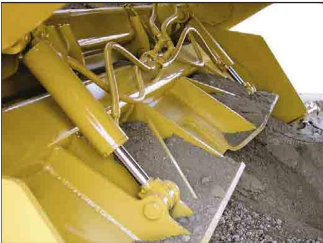
**Hydraulically operated front door.** Allows the operator to control the opening of the front door from the operator's station.
