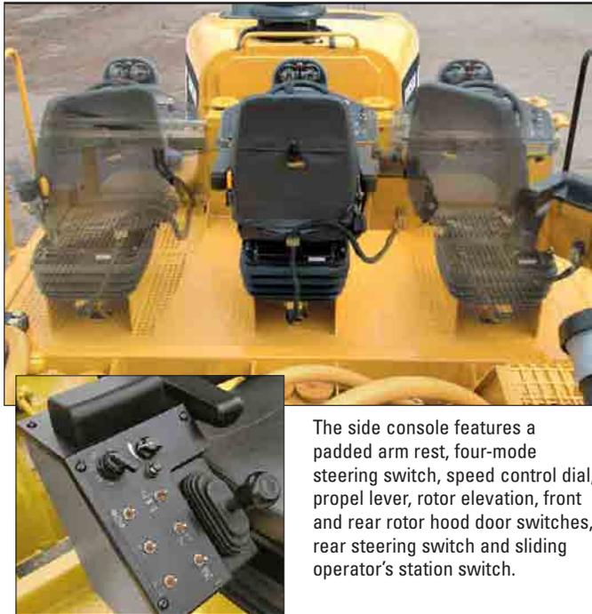
The side console features a padded arm rest, four-mode steering switch, speed control dial, propel lever, rotor elevation, front and rear rotor hood door switches, rear steering switch and sliding operator's station switch.
