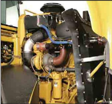
*Large one-piece fiberglass hood tilts forward for exceptional access to the engine and cooling package. Daily service points are accessible from ground level and are grouped on one side of the engine. Lower side panels open wide for even greater access.*
