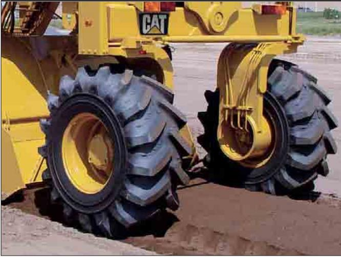
**Dual propel pump system.** One pump is dedicated to drive the front wheels, while the second propel pump is dedicated to drive the rear wheels.
