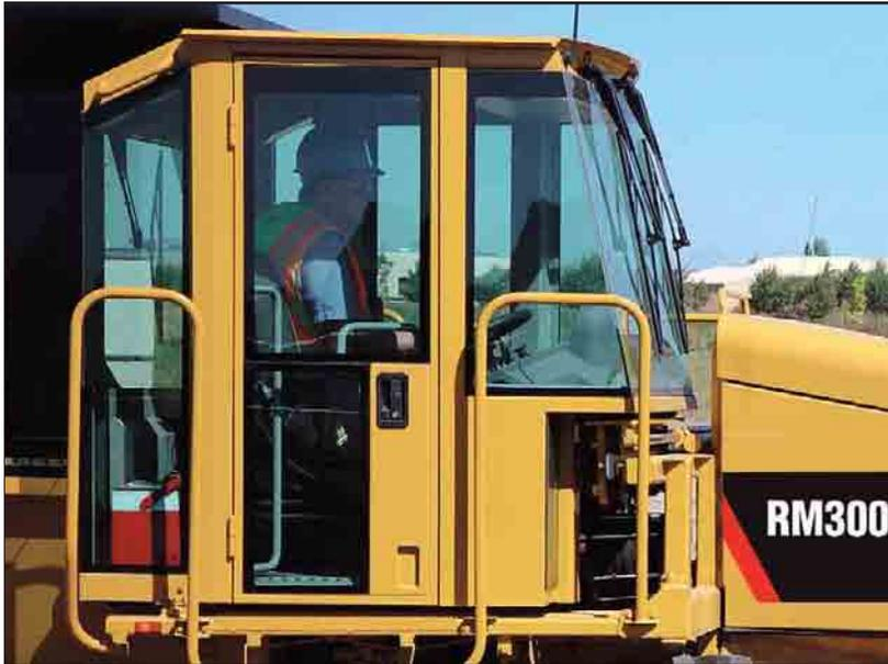
**Pressurized iso-mounted cab.** Maintains noise, dust and the elements out, and comfort in.
