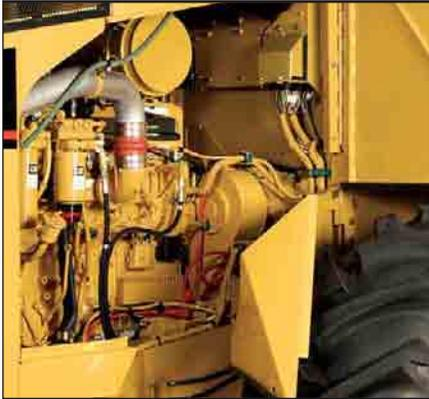
Daily service points are accessible from ground level and are grouped on one side of the engine. Hinged ground level side panels open wide for total access to engine components. Lower side panels can easily be removed for even greater access.
