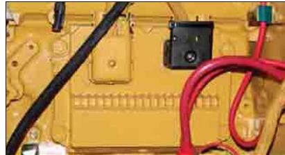
**C11 Cylinder Block.** The cylinder block is a one-piece, grey iron block that features generous ribbing for stiffness and heavy bearing bulkheads for rigidity and strength as the crankshaft turns. This new design supports the engine's higher compression ratios and increases its power density. The incorporation of straight-thread, o-ring connection points reduces the loss of engine oil and fluids.
