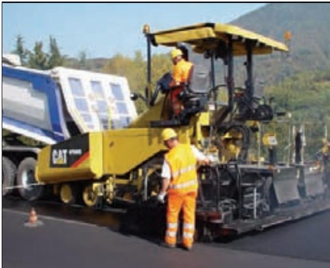
*The AS4251C screed paves from 2550 mm to 5000 mm. With mechanical extensions added to both sides, maximum paving width is 7000 mm (electric heat and LPG heat screeds).*
