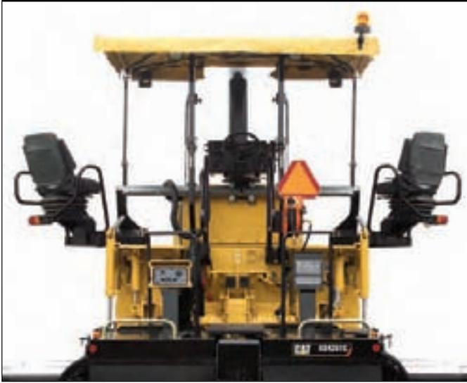
**Dual Operator's Station.** The ergonomic dual operator's station incorporates a sliding control console, ground speed indicators, adjustable suspension seats, armrests and retractable seat belts.
