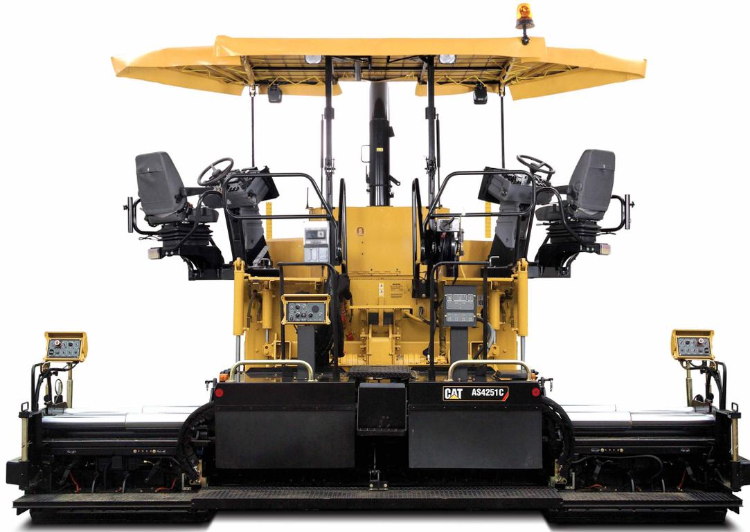
*Tamper bars combined with vibratory screed plates optimize mat density behind the screed.*
