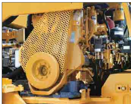
Large engine service doors provide optimum access to engine and hydraulic components from ground level.
