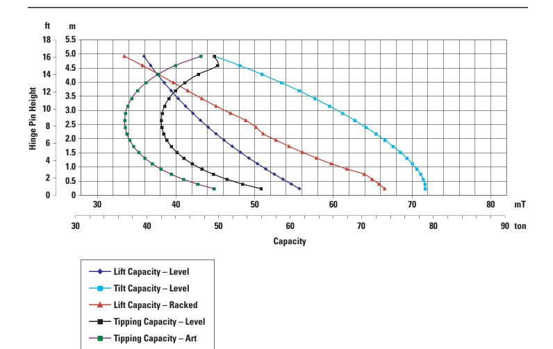
Performance curves shown above represent 988H (serial # BXY 4000 and up) machines equipped with the Block Handling arrangement with CWTS Quick Coupler and Block Fork for a 1.6 m (5.25 ft) block. Performance may be affected if the machine is configured with a different AEM attachment. Curves are shown at 100% of static ratings and should not be used to determine maximum machine load. Machine load ratings are determined by industry standards based on application and site conditions.
