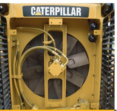
The engine radiator, Air To Air After Cooler (ATAAC), and hydraulic oil cooler are packaged in a single plane. Aluminum bar plate construction provides durability and allows for higher heat transfer and superior corrosion resistance. The standard cores feature 6 fins per inch to allow debris to pass through and reduce plugging concerns.
