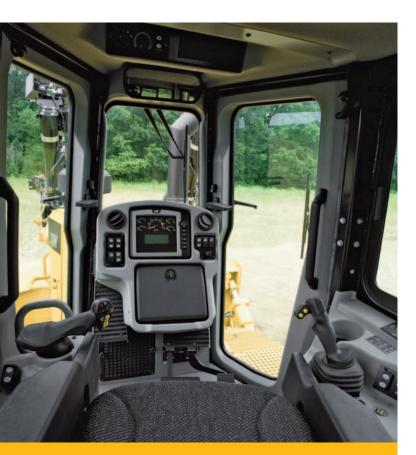
The D6T cab is designed and equipped for operator productivity, safety and comfort. An isolation-mounted cab reduces noise and vibration. Large single-pane windows, tapered hood and notched fuel tank provide excellent visibility to all sides of the machine and around the job site.
