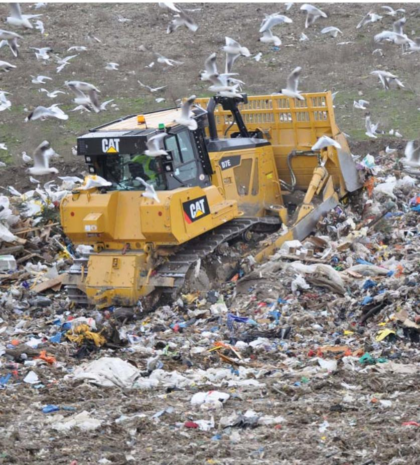
The D7E's structures are purpose built of high-quality steel and box section construction. When it comes to structures, Caterpillar is thorough, with application specific, finite element analysis at initial design, followed by prototype shake table testing, and finally pilot machine testing prior to production. The results are long-life structures built for loads associated with quick directional changes, extreme slopes and heavy-duty pushing or pulling.
