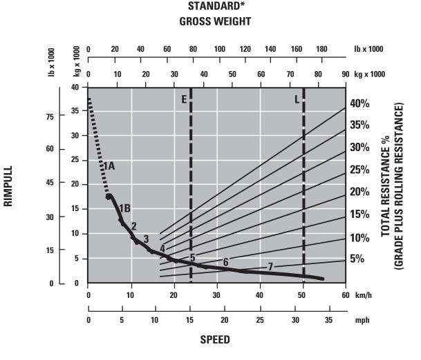
1A – 1st Gear (Converter Drive) 1B – 1st Gear (Direct Drive)
