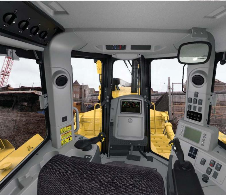
The D8T cab is designed and equipped for operator productivity, safety and comfort. Large single-pane windows, tapered hood and notched fuel tank provide excellent visibility to all sides of the machine and around the job site. New standard and optional light packages extend the productive work day.
