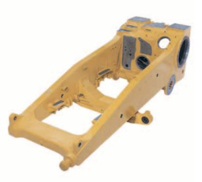
The D8T mainframe is built industry-leading tough – heavy steel castings, full box section frame rails and continuous rolled sections on top and bottom frame rails provide the strength to absorb high impact shock loads and twisting forces.
