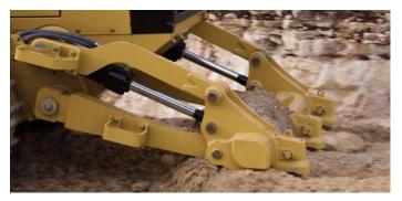
• **Ripper** – A 3-shank parallelogram ripper facilitates working in frozen ground and hard materials like asphalt, rocky ground and hard clay. Ripper shank options are available to help improve ripping productivity.
