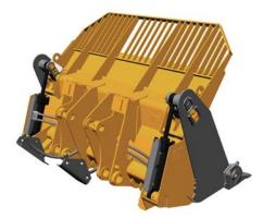
Multi Purpose Landfill bucket – has a capacity of 4.6 m<sup>3</sup> (6.0 yd<sup>3</sup>) and can greatly expand the 973D's versatility. It can act as a typical bucket for loading trucks, dozing waste or digging. It can also instantly change into a dozer-type blade for spreading cover material, or it can sort material with the ability to clamp on to debris. By adding the trash rack to this bucket, its capacity to doze and load material increased 53%.
