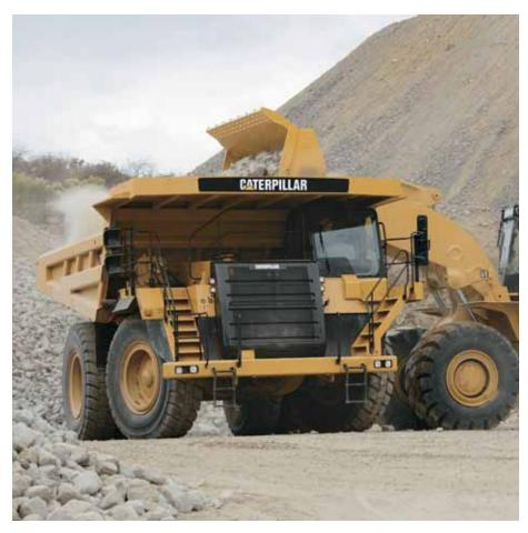
Overloading causes excessive wear on vehicle components, such as brakes, tires and drive train, reducing component life and increasing maintenance costs and repairs. Matched Systems. Designed to work as an optimum pass/match system, the 777F is best sized to match the Cat® 992K Wheel Loader, with a four to five pass/match, and the 993K Wheel Loader with four pass/match.
