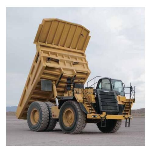
Cat Truck Bodies. Matching the truck body to the application is a critical part of achieving the best value from your 777F. Caterpillar offers a variety of application specific body options. The Caterpillar exclusive 10/10/20 payload guidelines help achieve a balance of excellent payload with safe operation.
