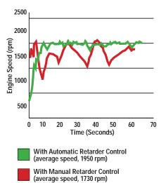
• Faster Speeds. ARC allows the operator to maintain optimum engine speeds for up to 15 percent faster downhill hauls and greater productivity.
