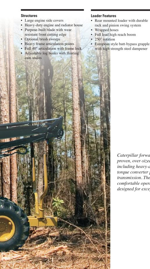
Caterpillar forwarders have proven, over-sized components including heavy-duty axles and torque converter power shift transmission. The spacious, comfortable operator station is designed for exceptional visibility.
