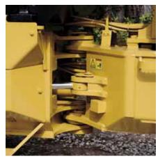
**Hitch**. A heavy-duty center section features oversized plates and bosses to disperse forces. A large double-tapered roller bearing is used on the lower hitch for reduced flexing stress and maintaining tight joints.
