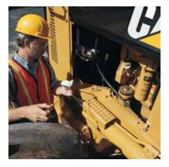
**Electrical System.** The 24V electrical system delivers dependable electrical power for engine cranking, additional lighting, and engine diagnostics. Wiring circuits are color coded, numbered and protected by circuit breakers.
