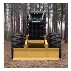
Decking Blade. The decking blade efficiently clears landings and roads, and maintains log decks. It features box section steel arms for superior strength and durability. Decking blade pusharms are mounted directly to the mainframe for excellent strength, and set lower and forward for efficient clearing of slash and debris as well as log deck maintenance. The electro-hydraulic control improves operator comfort and control of the decking blade.
