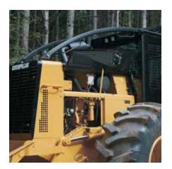
Ouick-Access Engine Doors. Large, hinged engine enclosure doors make regular maintenance as easy and fast as possible. Easy access to daily service points increases the likelihood that maintenance will be done, and increases machine service life. In addition, less maintenance time means more working time and greater productivity.
