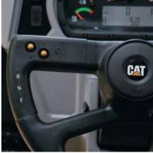
Machine Controls. The comfortable operator environment uses ergonomically designed and placed machine controls to reduce fatigue and increase productivity.
