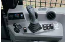
Auto-Grab Feature. Auto-Grab, engineered by Caterpillar, constantly monitors tong pressure and adjusts as needed to securely hold grapple loads while skidding. It is easily activated on demand by a switch located on the right-hand control lever.
