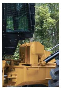
Hydraulic Winch. The 535C features an electronically controlled hydraulic winch for grapple applications, replacing the mechanical winch. The hydraulic winch improves application flexibility by allowing the tractive effort to be used while winching, and eliminating the continuously rotating driveshaft.
