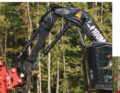
With up to 15,600 lb (7100 kg) of bare pin lift capacity at 20' (6.1 m) on the 532 track feller buncher, the 500 series machines are dominant over competitors in their size classes. With market leading lift capacity, 26.6' (8.1 m) of maximum reach, and tight stick tuck-in capabilities, these machines deliver high performance felling in all applications. The 532 track harvester delivers the same high performance with 9,100 lbs (4100 kg) of bare pin lift capacity and 32' (9.8 m) of maximum reach.
