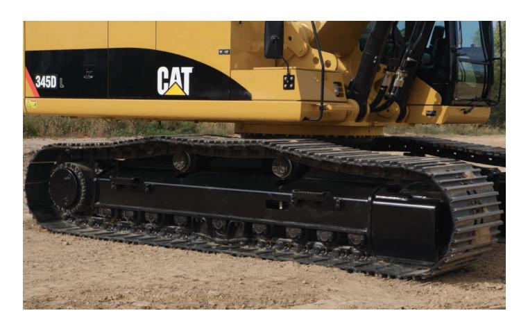
**Undercarriage Options.** Track with Positive Pin Retention 2 (PPR2) and cast idlers are available as attachments on the 345D L. The PPR2 prevents loosening of the track pin from the track link and the cast idler is designed for extended life. Both options are ideal for extreme applications or those that require a large amount of travel.
