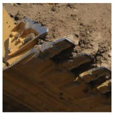
Caterpillar Ground Engaging Tools (GET). Caterpillar K Series<sup>TM</sup> GET is featured on the 345D L buckets. The K Series<sup>TM</sup> system uses a vertical retainer, which is easier to remove and install than the old Cat J Series pin. There are a variety of teeth, side cutters, and sidebar protectors to match operating conditions.
