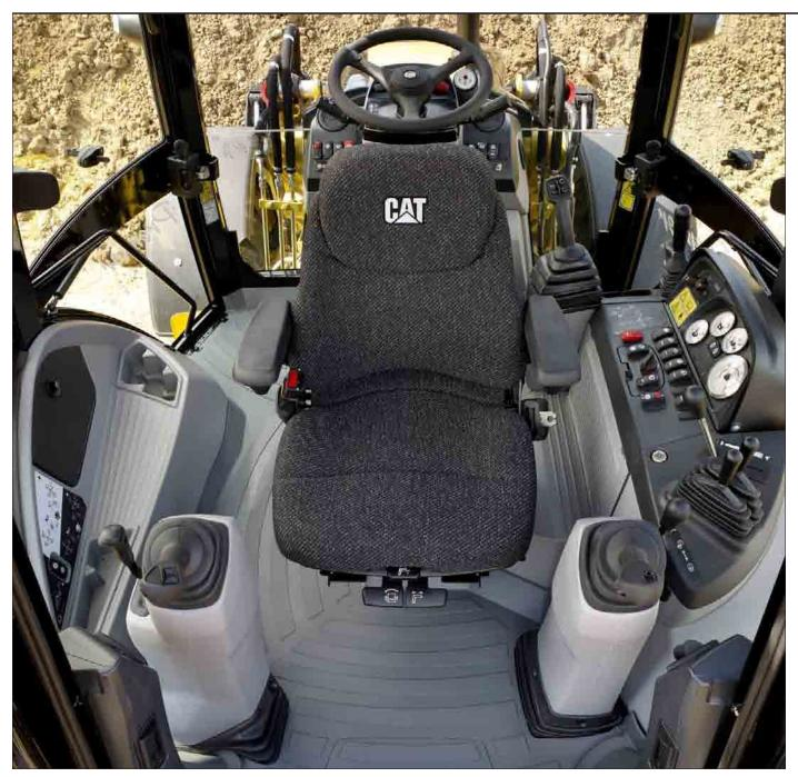
**The 444E Cab is Designed with Today's Operator in Mind** The E-Series cab is designed to provide maximum comfort, ease of operation, and overall style for today's demanding operator. The new design incorporates curved glass for improved interior space and visibility, and the cab is widened for better performance when turning from one mode of operation to the other. Cab comfort is enhanced with the firstclass Cat air suspension seat designed to reduce fatigue.
