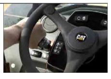
**Optional Auto-Shift Transmission**Work faster with the optional Auto-Shift transmission. The Auto-Shift transmission provides automatic shifting between five forward and three reverse gears. There is no floor mounted shift lever, so the operator has more floor space and better access through the right hand door.
