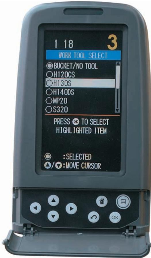
**Auxiliary Hydraulic Options.** Allows you to configure your 320D LRR to meet your work tools needs, while increasing its versatility.
