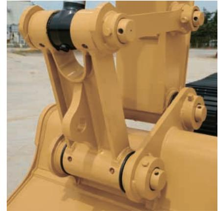
**Bucket Linkage.** The power link improves durability, increases machine-lifting capability in key positions and is easier to use than compared to the previous power link. Lifting from the power link lift eye gives you the optimum lift performance. It allows you to lower the load point, which maximizes the use of the boom cylinders.
