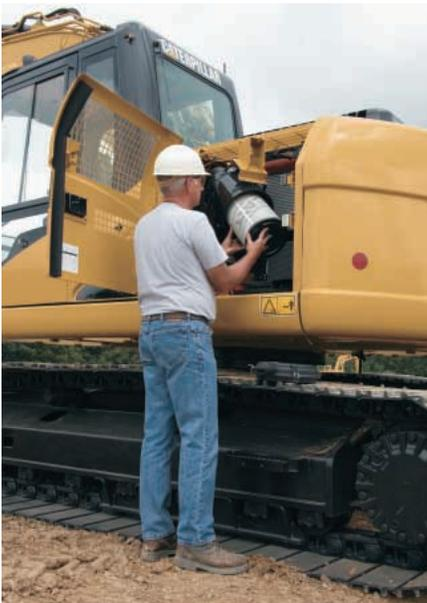
**Ground Level Service.** The design and layout of the 320D LRR was made with the service technician in mind. Many service locations are easily accessible at ground level allowing critical maintenance to get done quickly and efficiently.
