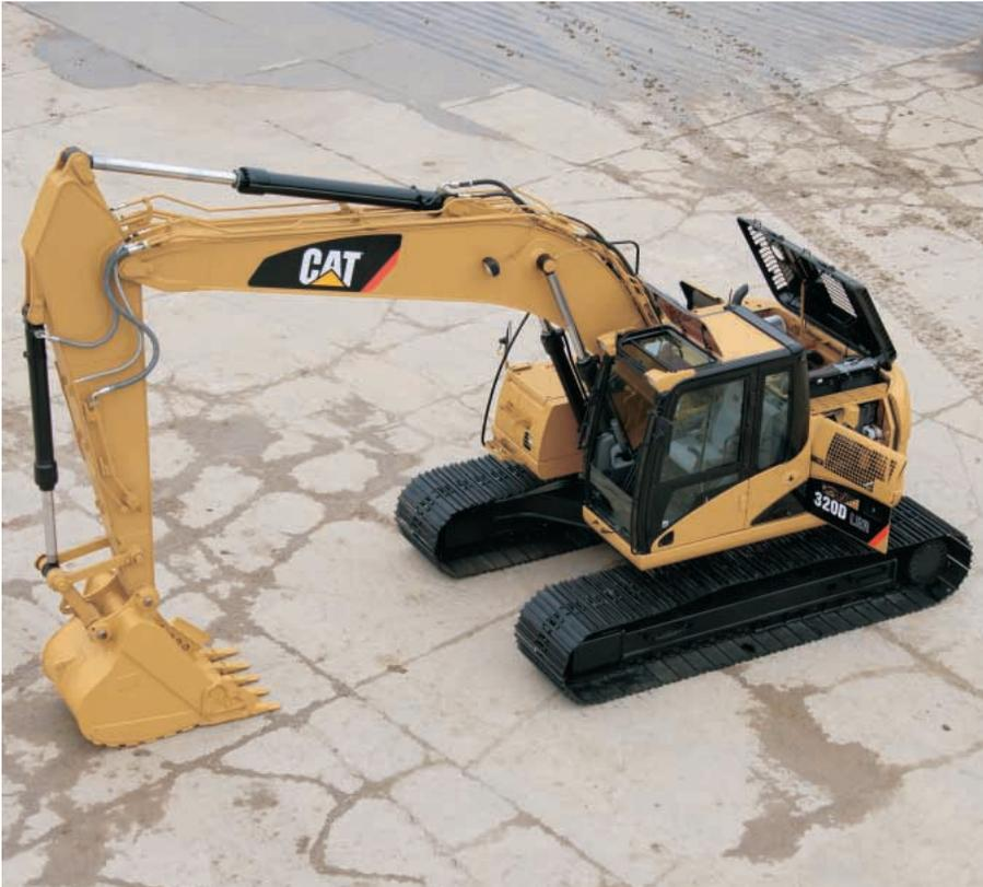
The air filter, the access point for the washer tank, and maintenance points for electric components, such as the battery, circuit breaker and controller, are positioned behind the cab, in the air cleaner compartment. The jump-start receptacle, which is an attachment, is near the battery. When equipped, the hand control pattern changer is located within this compartment.
