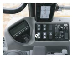
**Starting System.** The Electronic Speed Selector Switch (A), a "rocker" switch located on the right console, sets the engine rpm. The ADEM A4 engine controller will always start the engine in low idle. The engine rpm can be seen on the digital display of the instrument cluster in the gage cluster or in the performance menu in Messenger.
