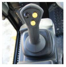
**Travel Speeds.** Travel speeds are infinitely variable between zero and top speed. Two speed modes "work" and "travel", provide two different speed ranges to best match machine speed and torque to the job conditions for maximum productivity. Maximum travel speed is 10 kph (6.2 mph) when the switch is set in the travel position.
