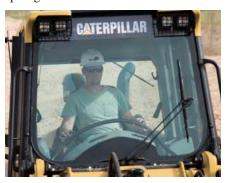
**Viewing Area.** Large windows use tinted glass to reduce glare and provide an excellent view to the bucket, tracks, and around the engine enclosure to the rear. Side windows slide top down to allow the operator to let fresh air into the cab and communicate.
