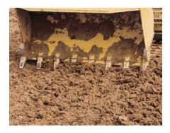
**General Purpose Bucket.** The General Purpose (GP) bucket is designed for excellent loadability and long life in a broad range of applications such as hard bank excavating, stripping and stockpile loading. High-strength, low-alloy steel helps the bucket resist dents and abrasions.
