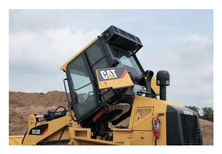
**Tiltable Cab.** The 953D is equipped with a tiltable cab. This feature makes the maintenance and the repairs easier. By tilting the cab, you can access to the drive train and perform complete service of the hydraulic system.
