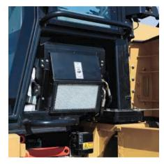
**Cab Air Filter.** The cab air filter, the grouped pressure taps, the cab tilt locking bar, the optional tilt cylinder and the tool box are conveniently located below the left-side cab window.
