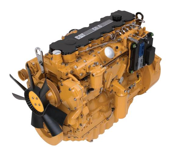
Cat C6.6 ACERT™. The Cat® C6.6 is a 6.6 liter (403 in³) displacement, six-cylinder, in-line configured engine that utilizes the Caterpillar® Common Rail fuel system for fuel delivery. It uses ACERT™ Technology, a series of Caterpillar engineered innovations that provide advanced electronic control, precision fuel delivery and refined air management, resulting in outstanding performance and lower emissions.
