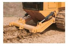
**Ripper-Scarifier.** A radial ripper-scarifier is available for the 953D as an attachment. It is mounted with two pins pressed into each side of the main frame. Two cylinders raise and lower the ripper. The ripper beam has three pockets for holding ripper shanks. The six pins in the linkage do not require lubrication.
