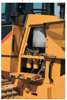
**Left side compartments.** Left engine compartment includes two spin-on hydraulic oil filters that provide filtration for the hydrostatic system.
