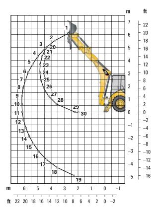
Lift Capacities are over-end values. Machine equipped with 4WD, OROPS, 1.00 m³ (1.31 yd³) general purpose bucket, and 116 kg (255 lb) counterweight. Extendible stick includes 488 kg (1,075 lb) counterweight.
