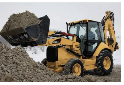
Caterpillar offers a choice of single tilt or integrated toolcarrier (IT) loader linkage to suit your application requirements. The IT loader controls provide single lever proportional control and fine modulation of the hydraulic work tools. A thumb roller operates auxiliary hydraulic functions such as the multi purpose bucket on the IT machines.
