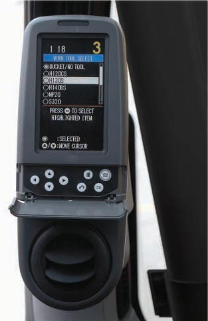
**Tool Control System.** The optional tool control system maximizes work tool productivity by configuring hydraulic flow, pressure, and operator controls to match a specific work tool. System versatility enables a wide range of tools to be used.
