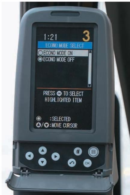
**Monitor.** The monitor is a full color 400x234 pixels Liquid Crystal Display (LCD) graphic display. The monitor angle can be adjusted to minimize sun glare and has the capability of displaying information in twenty-seven different languages.
