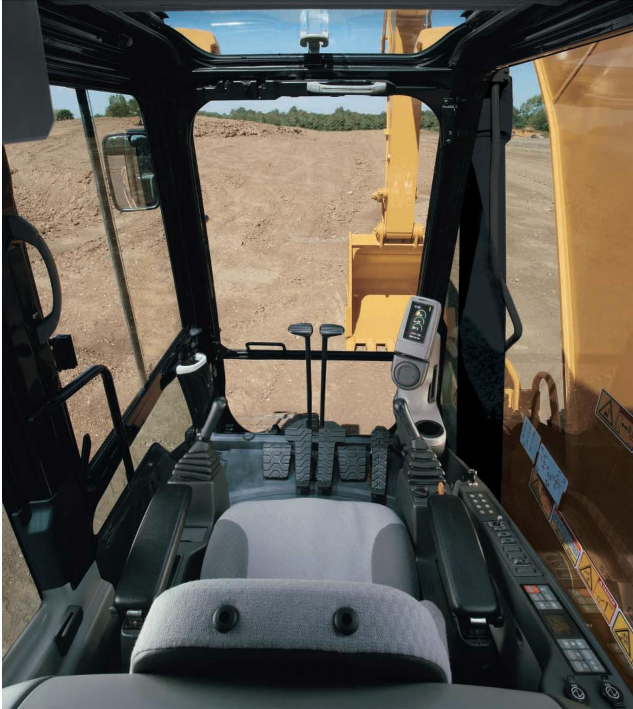
**Operator Station.** The workstation is spacious, quiet and comfortable, assuring high productivity during a long workday. The air conditioner and attachment switches are conveniently located on the right-hand wall, and the key switch and throttle dial are on the right-hand console. The monitor is mounted in front of the right front cab post and is easy to see.
