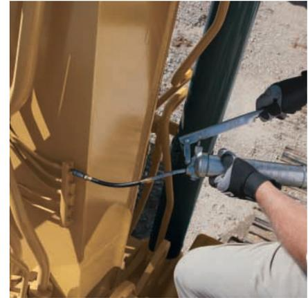
**Greasing Points.** A concentrated remote greasing block on the boom delivers grease to hard-to-reach locations on the front.
