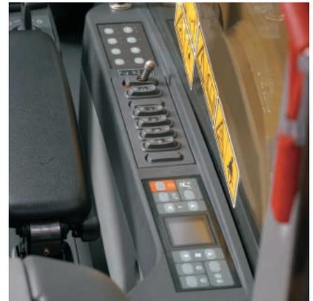
**Console.** Redesigned consoles feature a simple, functional design to reduce operator fatigue, ease of switch operation and excellent visibility. Both consoles have attached armrests with height adjustments.
