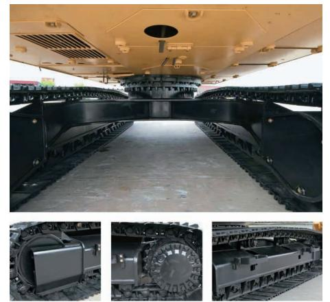
**Rollers and Idlers.** Sealed and lubricated track rollers, carrier rollers, and idlers provide excellent service life, to keep the machine in the field longer.
