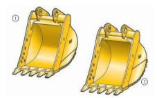
(1) Heavy-Duty Buckets. Heavy-duty (HD) buckets are used for a wide range of moderately abrasive applications such as mixed dirt, clay and rock. HD buckets have best loading and dumping characteristics and will empty easier in cohesive material. More robust construction than the GP buckets.
