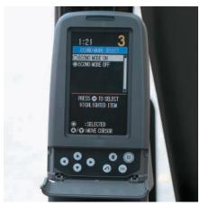
**Monitor.** The monitor is a full color 400x234 pixels Liquid Crystal Display (LCD) graphic display. The monitor angle can be adjusted to minimize sun glare and has the capability of displaying information in Chinese and twenty-six other languages.
