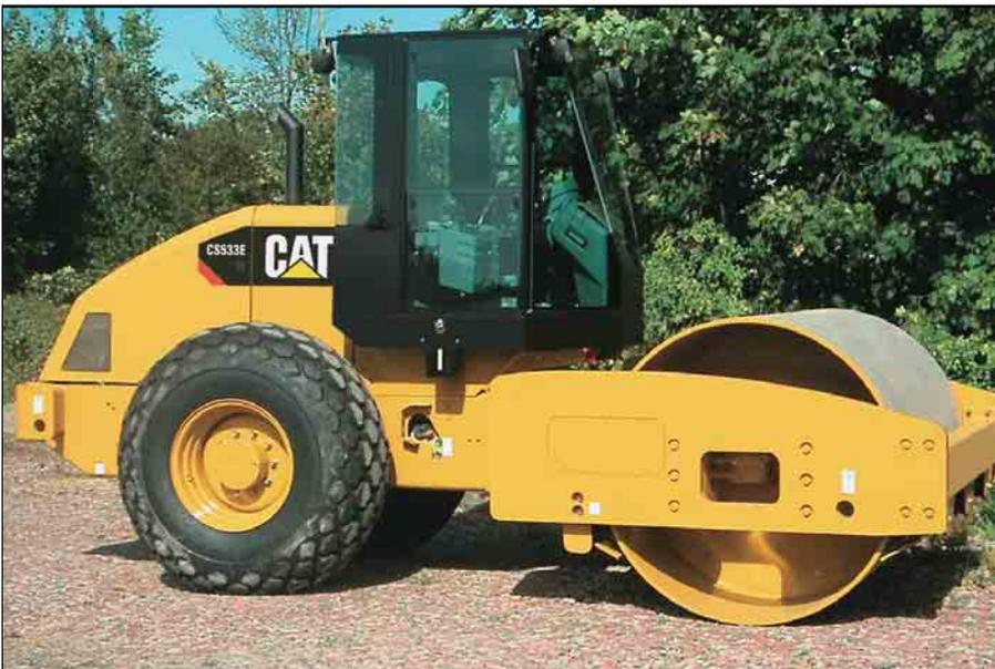
**Increased machine weight.** The operating weight is approximately 1500 kg heavier than the standard CS533E. When equipped with this option the CS533E Heavy Weight competes in the 12 to 15 metric ton size class.
