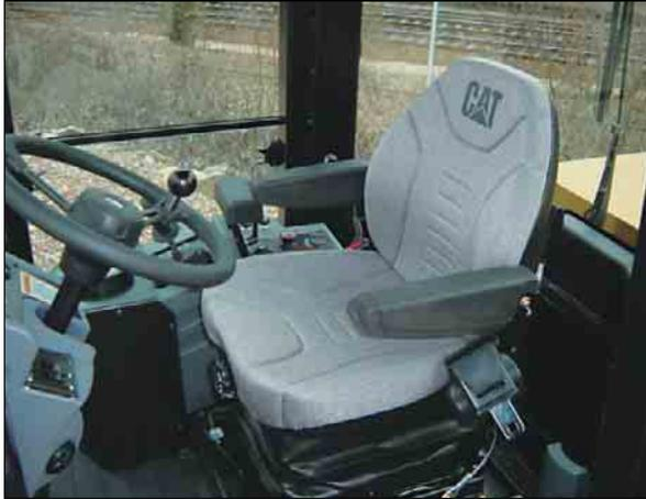
**Single lever control.** The single lever control for propel and vibratory On/Off provides simple and low effort operation. A padded adjustable wrist rest provides comfort.
