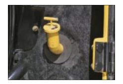
With the hood closed, quick checks of engine oil level and the coolant sight gauge can be completed through the side service doors.
