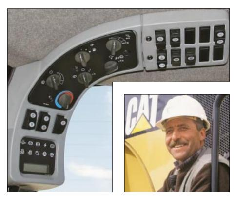
**Controls.** The main control panel on the 972H is located high on the right ROPS post – keeping everything within reach of the operator while maintaining visibility to the ground. Keeping all switches and controls conveniently placed allows better operator efficiency and improved productivity, while minimizing operator fatigue.
