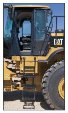
Entry and Exit. A ladder with selfcleaning steps keeps debris build-up to a minimum. The ladder is at a 5° forward incline for easy entry and exit. Platforms are wide allowing ease of movement to the front or rear of the machine. The main cab door opens a full 180° and latches in place to allow safe navigation to the rear of the machine. The right side door opens 10°, or completely for secondary exit simply by pulling a pin. A full-length ladder on the right side facilitates safe exit if needed.
