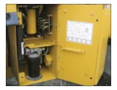
**Hydraulic Service Center.** Transmission oil and hydraulic oil filters are located in the Hydraulic Service Center, behind the hinged, right-side access ladder. The hydraulic oil tank can be drained from this location using the access port.
