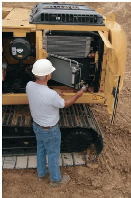
**Radiator Compartment.** The air conditioning condenser swings out to allow access to the engine radiator and oil cooler. The air to air after cooler is fixed in position above the condenser.
