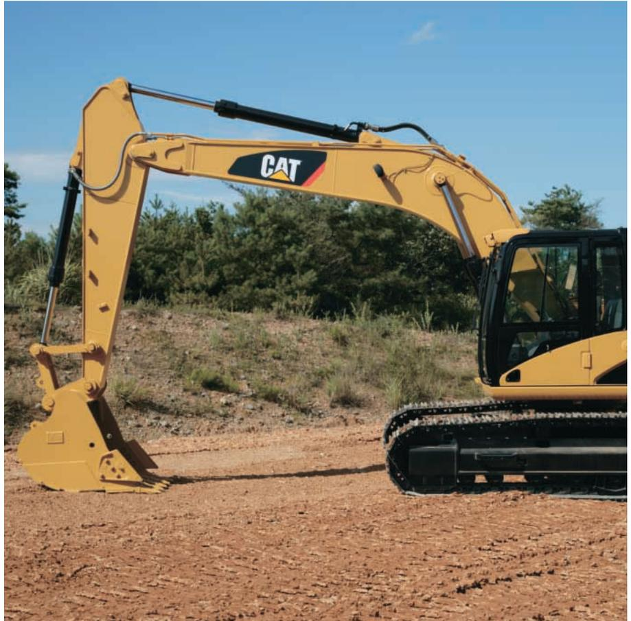
**Linkage Pins.** The bucket linkage pins for the Mass Excavator configuration have been enlarged to improve reliability and durability. All the pins in the front linkages have thick chrome plating, giving them high wear and corrosion resistance.
