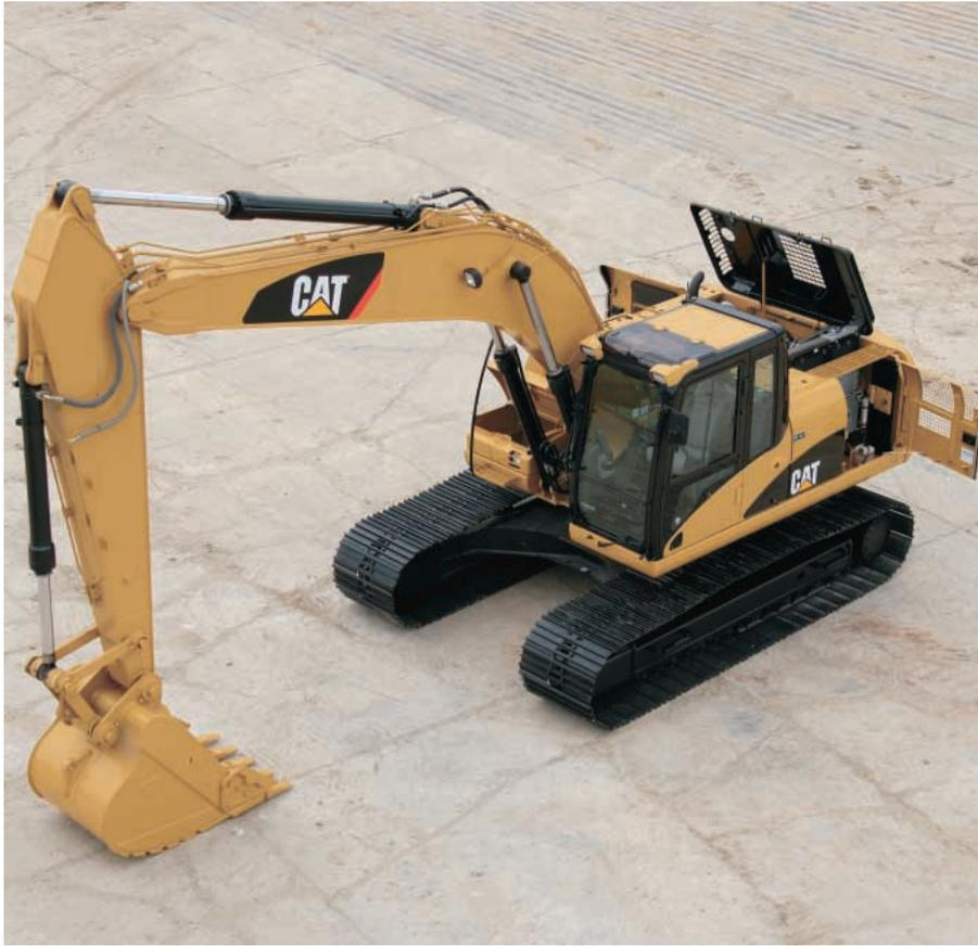
**Ground Level Service.** The design and layout of the 320D was made with the service technician in mind. Many service locations are easily accessible at ground level allowing critical maintenance to get done quickly and efficiently.
