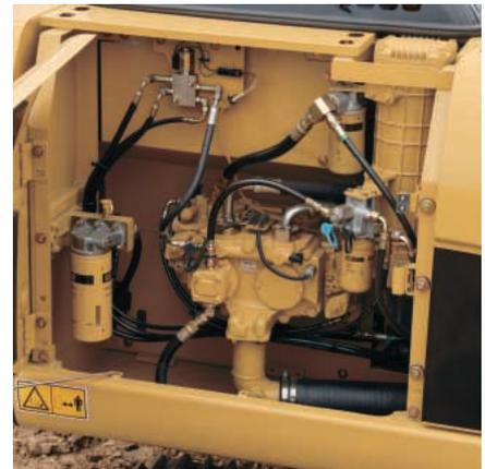
**Diagnostics and Monitoring.** The 320D is equipped with S•O•S<sup>SM</sup> sampling ports and hydraulic test ports for the hydraulic system, engine oil, and for coolant. A test connection for the Cat Electronic Technician (Cat ET) service tool is located in the cab.
