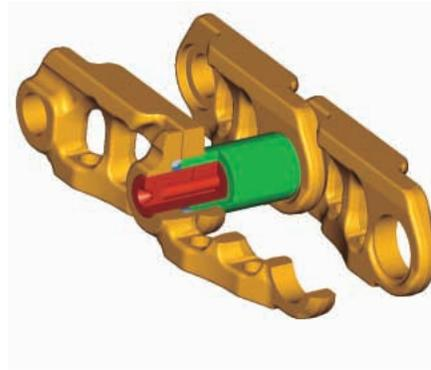
**Track.** The 365C L comes standard with the new grease lubricated track called GLT4. The track links are assembled and sealed with grease to decrease internal bushing wear, reduce travel noise and extend service life lowering operating costs.
