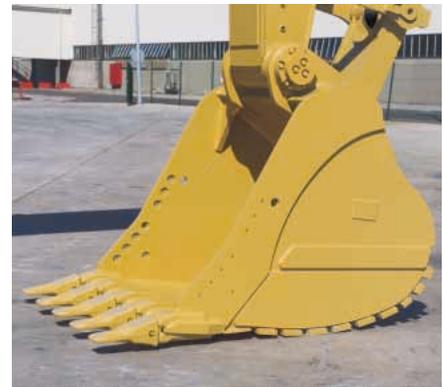
**Ground Engaging Tools.** Caterpillar Ground Engaging Tools (GET) include a variety of side cutters, sidebar protectors, and tip options to match operating conditions.
