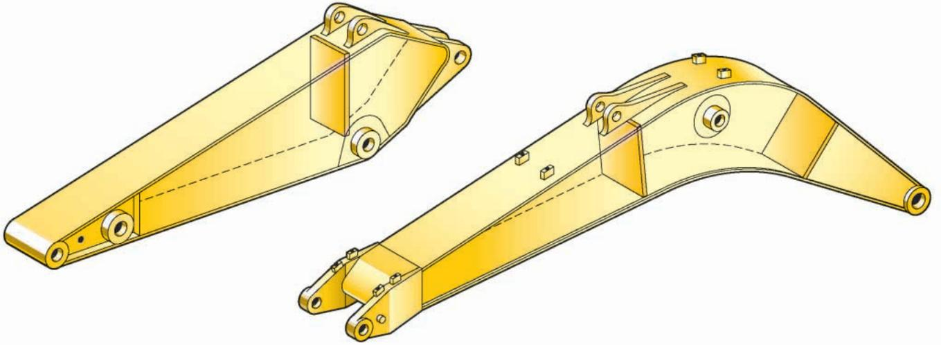
**Front Linkage Attachments.** Select the right combination of front linkage with your Cat dealer to ensure high productivity from the very start of your job. Two types of booms and six sticks are available, offering a range of configurations suitable for a wide variety of applications. The 365C L offers a large combination of reach and digging forces for optimum versatility.
