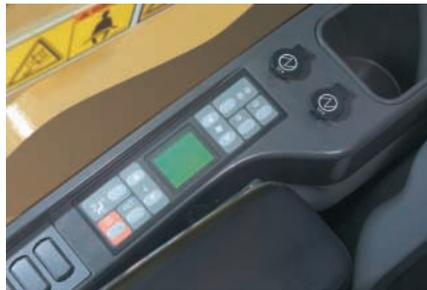
**Consoles.** Redesigned consoles feature a simple, functional design to reduce operator fatigue, ease of switch operation and excellent visibility. Both consoles have attached armrests and allow the height of the armrests to be adjusted.
