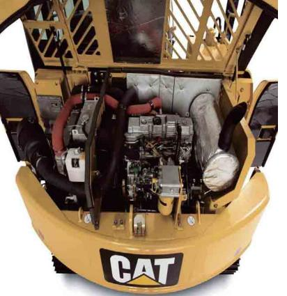
Robust, reliable and easily serviced are the key attributes of Caterpillar Mini Hydraulic Excavators. Full steel body work panels provide durable protection against damage. All daily service points are easily accessed through the rear hood and side cover and a 500 hour engine oil change period lowers operating costs. The Cat S•O•S. points assist easy oil sampling for preventative maintenance checks.
