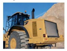
**New Hood.** A new hood has been designed for the 980H. Two layers thick, the new hood provides improved durability while maintaining visibility to the ground. The reinforced hood is more resistant to wind and mud build-up. The actuation system has also been improved. Electrohydraulically activated twin lift cylinders significantly reduce lift and lower time.
