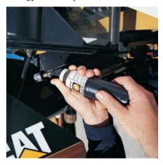
**S-O-S Fluid Sampling.** Oil sampling valves allow quick access to engine, transmission and hydraulic oils for S-O-S analysis. Sampling ports for steering, transmission, and brakes are grouped in lockable service compartments behind the cab. The S-O-S program enables problems to be detected before they occur and allows more convenient scheduling of service.
