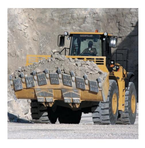
Steel Mill Applications. The Steel Mill Arrangement gives the added protection needed for extended life and lower operating costs in this rugged environment. The arrangement includes steel guarding for critical components, an extreme service transmission, heavy-duty engine and transmission mounts, hydraulic hose protection, insulated battery mounting, remote engine shutdown, remote parking brake release, transmission override, steel cable ladder, steel command control
