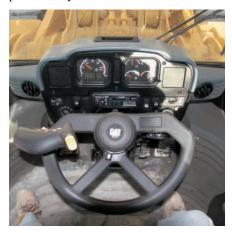
**Command Control Steering.** Reduce steering movements by a factor of 14 with Command Control Steering as compared to conventional steering. A conventional steering wheel requires two to three 360° turns to complete one turn of the loader – the Command Control wheel moves ±70° with only 26 N (6 lb) steering pressure to complete a turn – reducing operator fatigue.
