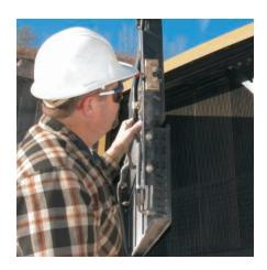
**Cooling.** The Next Generation Modular Radiator (NGMR) cores are a modular design permitting replacement of a single core without removing the entire radiator – reducing repair costs and downtime. A sight gauge located on the shunt tank allows quick service checks. The perforated, corrugated grill swings out for easy access to the cooling cores.
