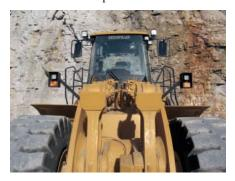
**Structures.** The 980H retains the same basic structures as the 980G Series II. Full box section engine end frame absorbs shock loads and twisting forces while supporting the drive line for rigid component alignment. The frame is over 90 percent robotically welded providing deep weld penetration for maximum durability and fatigue strength.
