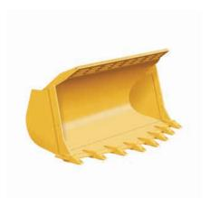
**Rock Buckets.** Rock buckets are designed for face or bank loading in mining or quarry applications. The straight-edge rock bucket provides higher breakout force and increased dump clearance. The spade-edge rock bucket offers better penetration.
